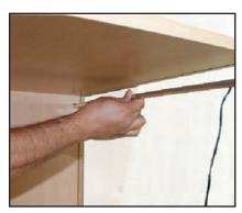
**Step 5.** Align aluminum pole to end of light bar and mark hole placement on base.
